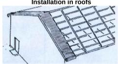
Starting at the end of the roofing framework, measure the length across the trusses, adding enough to allow overhang at both ends. Cut the first piece and lav in place. Pull tight from both ends and attach to trusses or purlins using self-tapping screws and washers or with pressure-sensitive reflective tape. Cut the second length, laying parallel to first. Make sure to butt or slightly overlap edges.
