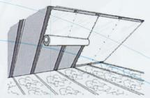
Staple solid R+HEATSHIELD from the ridge board down the eave or horizontally across the rafters, whichever is easier. If ridge venting is used, leave a 2" opening below the ridge board and above the floor joists as shown to prevent trapping heated air. Never block any venting with R+HEATSHIELD.
