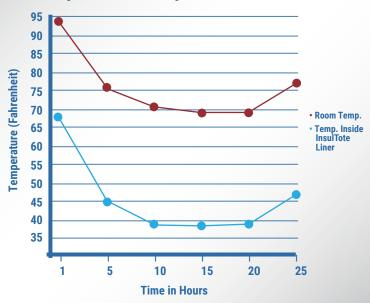
Testing was conducted in a controlled environment using a standard corrugated box lined with an InsulTote insulated box liner. Items placed inside the liner were (12) 4.25 oz candy bars and (4) coolant bricks.
